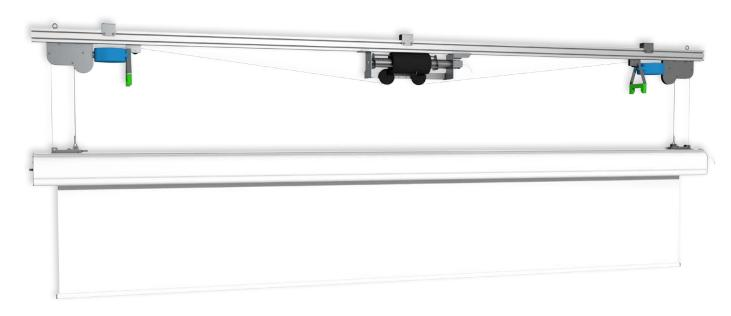
This **SCREEN WINCH SYSTEM** for **MAJOR PRO-C** is a particular lift that enables to lower until 7 mt. electrical screens from 500 cm. to 700 cm. of width. The Screen Winch is supplied with a manual on/off switcher but can be also ordered with a double channel RF remote control with external recevers. A **SAFETY DEVICE** is built-in, in order to offer maximum security in case of any failure of the mechanism.
