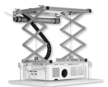
The PROJECTOR LIFT SI-H L 100 is studied in order to support large and heavy video projectors up to 30 Kg. of weight. The SI-H L 100 is supplied with an extremely silent motor that allows a descent from a minimum of 15,5 cm. to a maximum extent of 97 cm.
